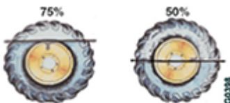
Fig. 2 Level, filling tyres with fluid
