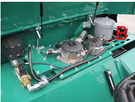
Fig. 33 Replacement of off-line filter, hydraulic oil
