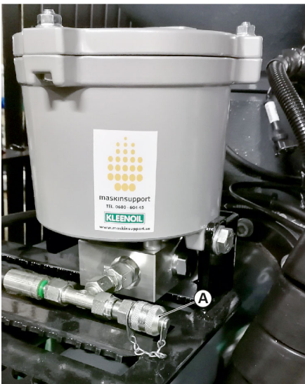
Fig. 30 The outlet is located next to the hydraulic system's off-line filter.
