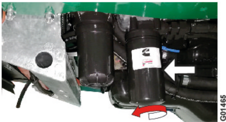
Fig. 14 Removal of old oil filter
