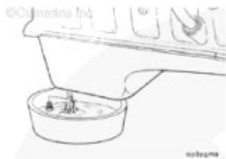
Fig. 10 Removal of oil drain plug
