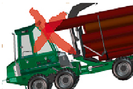
Fig. 114 Loading over the top of the gate
