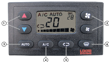
Fig. 152 Air conditioning, panel
