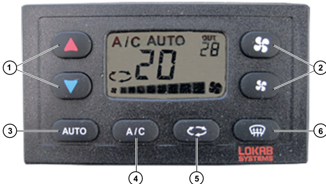
Fig. 50 Control panel for air conditioning system
