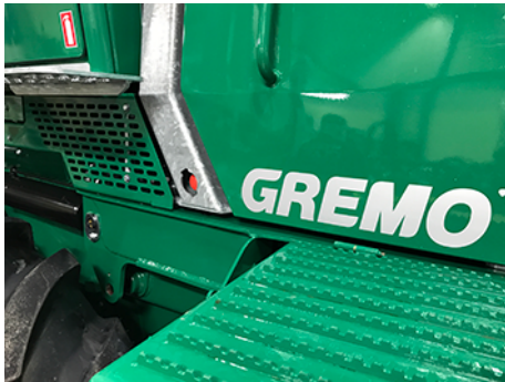
Fig. 10 External emergency stop
