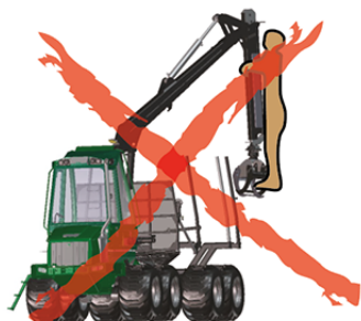
Fig. 21 lifting people with crane
