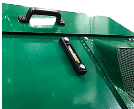
Fig. 94 Hydraulic tank sight glass
