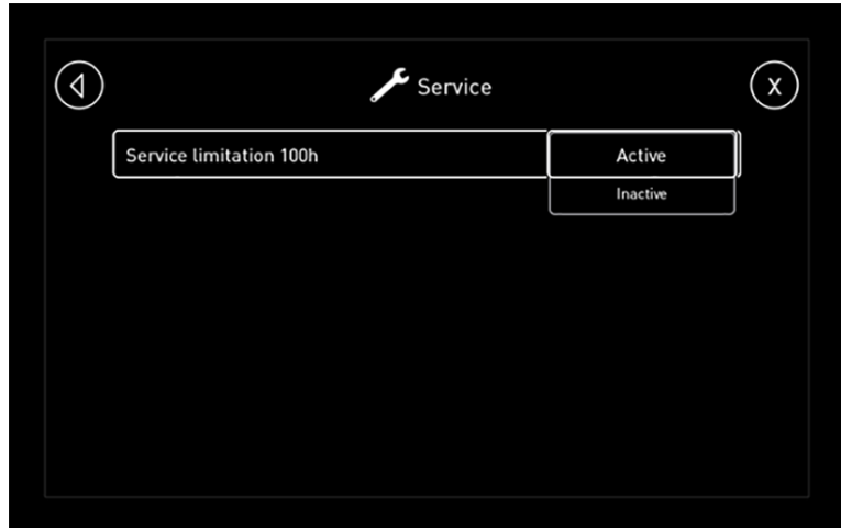
Fig. 77 GreControl, Limitation activation
