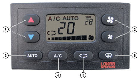
Fig. 144 Air conditioning, panel
