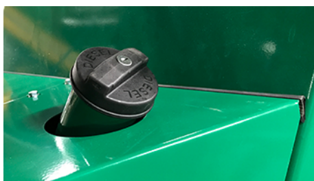
Fig. 122 Fuel filling line
