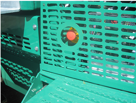
Fig. 10 External emergency stop
