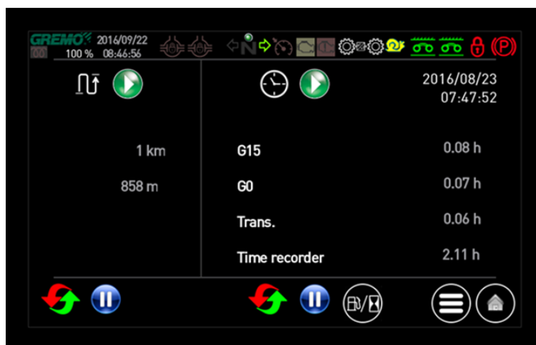
Fig. 67 GreControl, operation monitoring window
