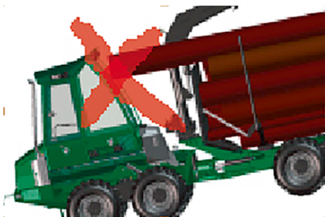
Fig. 112 Loading over the top of the gate
