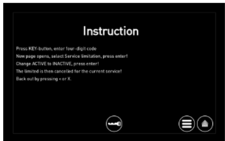
Fig. 72 GreControl, service code info
