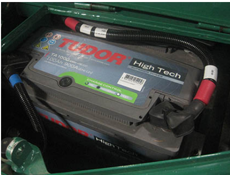
Fig. 134 Batteries in the right branch deflector
