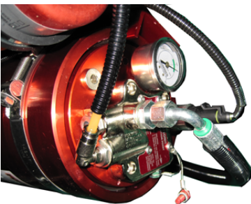
Fig. 149 Fire extinguishing system, safety screw
