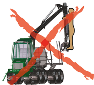
Fig. 19 lifting people with crane
