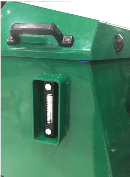
Fig. 92 Hydraulic tank sight glass
