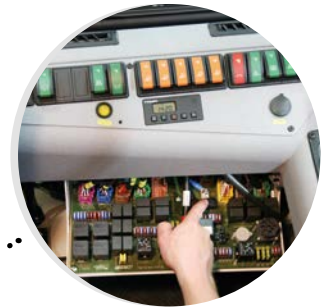
Circuit board in the cab for power supply.
