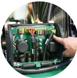
Circuit board in engine space for power supply
