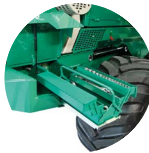
Heating of storage compartment and tools in the left front part of the chassis.
