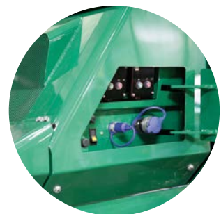
Connections with quick connectors and switches to diesel and hydraulic oil
